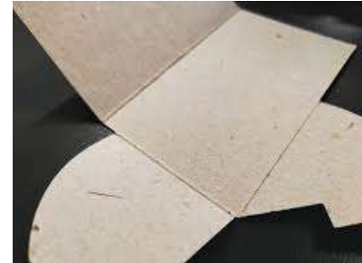
Recycled board with functional barrier
